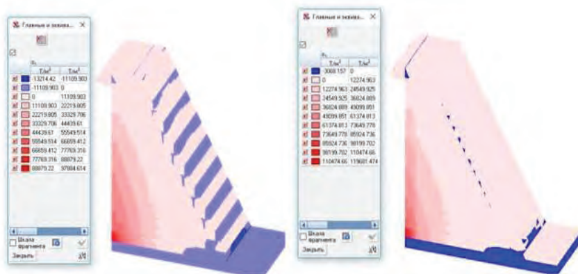
Picture 2 – The stresses in the dam (on left – reinforced concrete, on right – fiber concrete)
