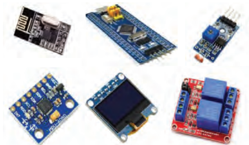
Fig. 2. The hardware modules used in the system, including (1) wireless communication module, (2) microcontroller core board, (3) photosensitive sensor module, (4) inertial measurement unit, (5) OLED and (6) relay control module
