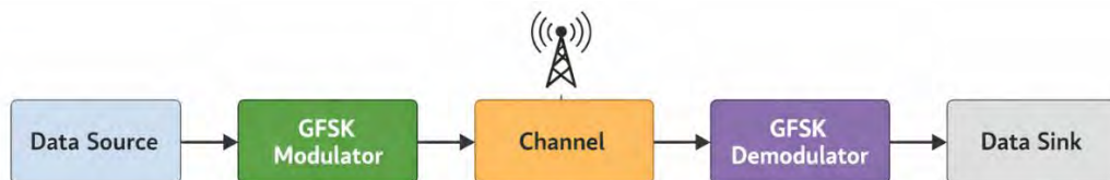
Figure 1 – Block diagram of the proposed GFSK-based UAV communication system
