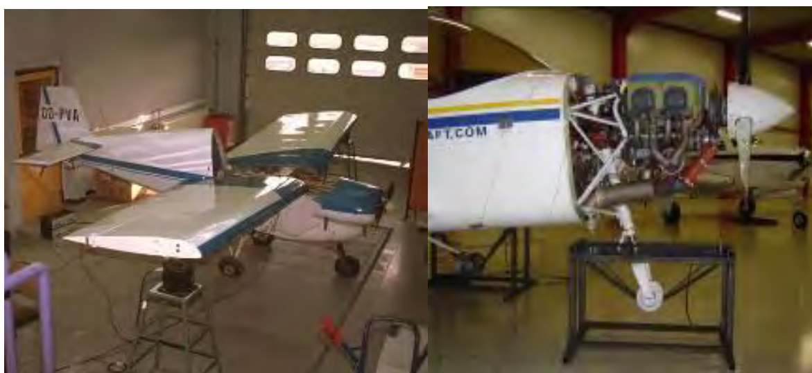
Figure 3 – Aircraft input excitation using a vibration exciter and isolation from external vibration sources
